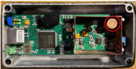
Fig. 3. TRNG with PIN diode (in red circle)
