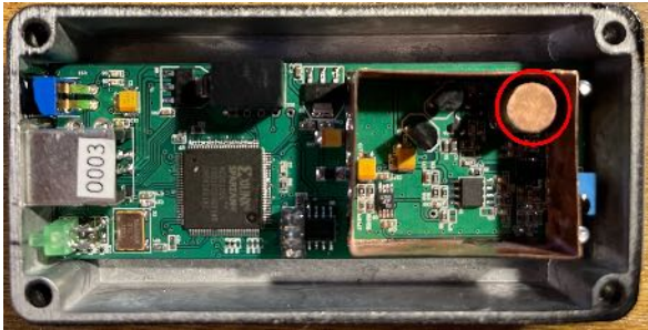
Fig. 3. TRNG with PIN diode (in red circle)
