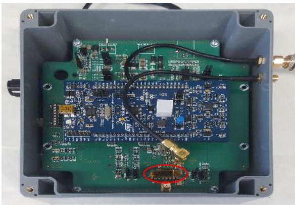
Fig. 4. TRNG with SPAD diode and quenching circuit module (in red oval)
